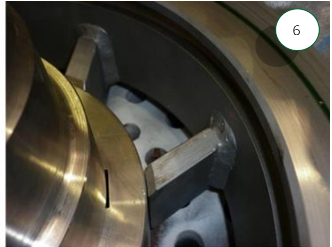
5. The new design external PE Endbell support is manufactured with a thread size that corresponding to the outer hub as per photo 4.
