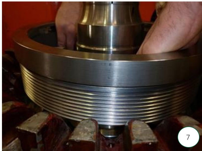
6. The new design external PE Endbell support is threaded and locked into the original outer hub.
